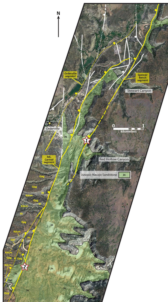
Figure 3. Simplified structural map of the steeply WNW-dipping central Sevier fault zone. Yellow faults represent the primary segments of the fault zone, and the white faults are subsidiary faults that help accommodate extension across the fault network. The green shaded areas represent exposures of the Jurassic Navajo Sandstone, and outlined areas labeled with yellow abbreviations are lithologies in the hanging wall of the Mt. Carmel segment, including: Kt (Cretaceous Tropic Shale), Kdcm (Cretaceous Dakota and Cedar Mountain Formations), Qag (older alluvial gravels), and Qal (modern alluvium). The white stars represent the locations of field and modeling studies performed by Pierce Hayton (1) and Morgan Sharp (2). Demi Durham focused her modeling investigation on the region north of the tip of the Spencer Bench segment.
