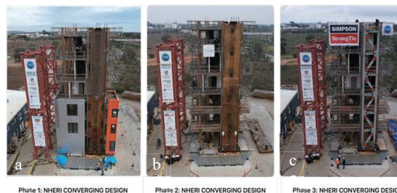
Figure 2: (a) Phase 1: Rocking walls with UFPs, (b) Phase 2: Rocking walls with BRBs, (c) Phase 3: steel Moment Frame with Yield Link Connectors.
