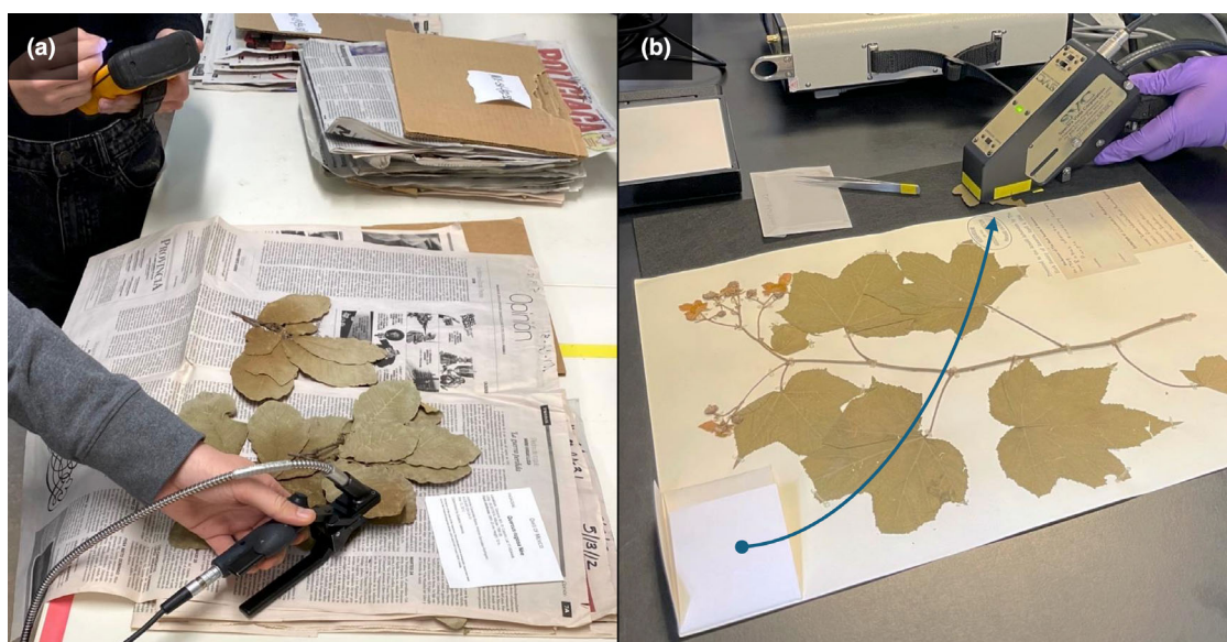
Fig. 1 Spectral measurements of pressed (a) and herbarium (b) leaf specimens. Pressed leaves (a; photograph by J. Cavender-Bares) are unmounted and easily scanned, while herbarium specimens are mounted and more variable in preservation. In (b), a detached leaf fragment from the packet is measured on a black background to avoid spectral interference (specimen from A: Herbarium of the Arnold Arboretum of Harvard University; photograph by D.M. White).
