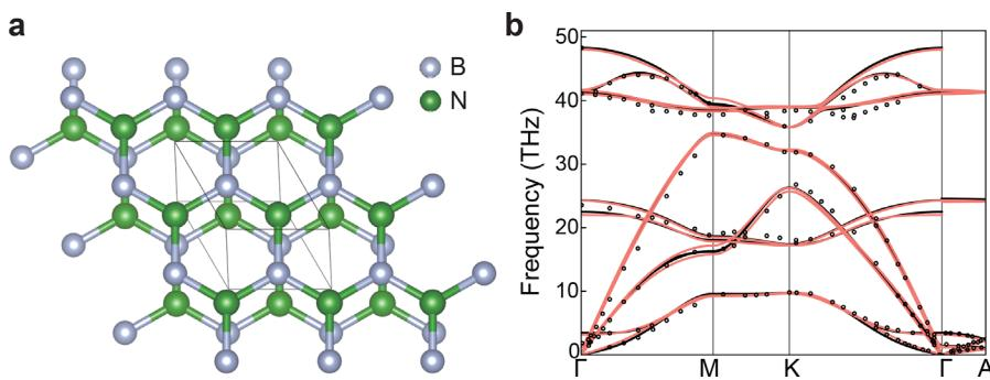
**FIG. 1.** Lattice structure and phonon dispersion of bulk h-BN. (a) Lattice structure of h-BN from a perspective view. The black wireframe shows one unit cell. (b) The phonon dispersion of bulk h-BN calculated with (red lines) and without (black lines) phonon renormalization at 300 K compared with the experiment<sup>49</sup> (black dots).
