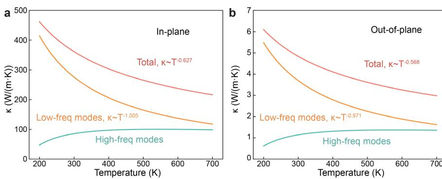
**FIG. 4.** Thermal conductivity contribution from high- and low-frequency phonon modes. (a) In-plane direction. (b) Out-of-plane direction.
