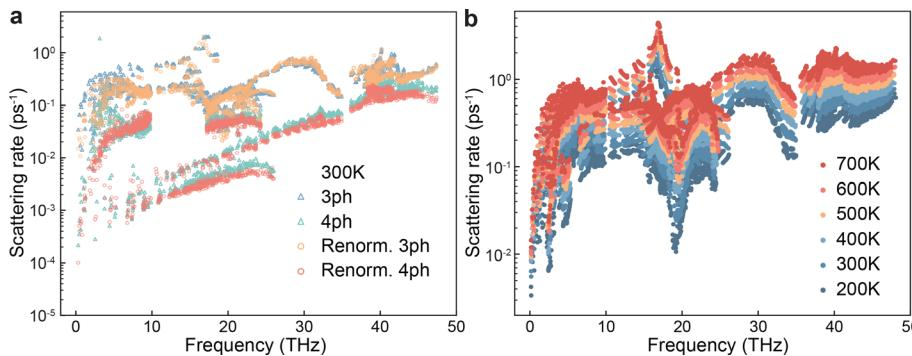
**FIG. 3.** Phonon scattering rate as a function of phonon frequency. (a) The 3ph and 4ph scattering rates at 300 K. Circle and triangle dots represent the scattering rates calculated with and without phonon renormalization at 300 K, respectively. (b) Temperature evolution of phonon scattering rates considering 3ph scattering, 4ph scattering, and phonon renormalization.
