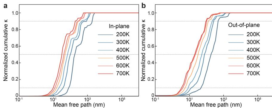
**FIG. 5.** Normalized cumulative thermal conductivity of h-BN as a function of phonon mean free path from 200 to 700 K. (a) In-plane direction. (b) Out-of-plane direction. The three dash lines stand for 10%, 50%, and 90% of total thermal conductivity, respectively.
