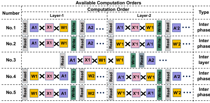
Fig. 8. Available GCN computation orders for reusing intermediate results when considering the data dependency of both intra- and inter-layer.
