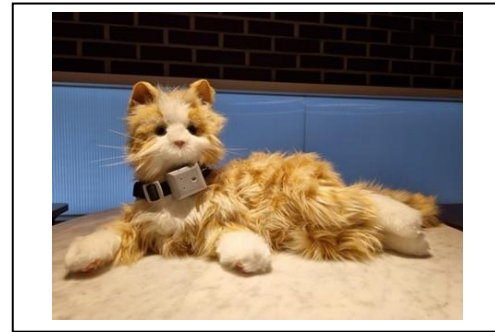
Figure 1. Robot cat wearing sensor collar
