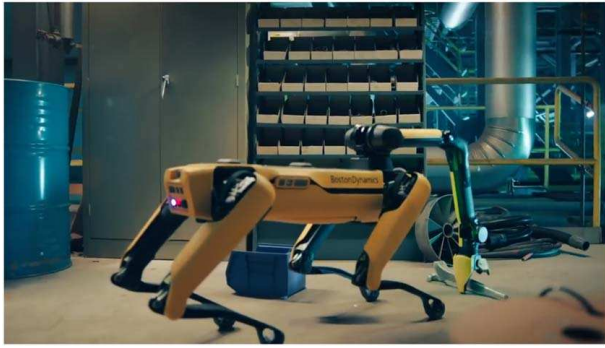
Fig. 1 State-of-the-art six-DoF robotic arm mounted on Boston Dynamics Spot. The arm weighs 8 kg and, when mounted on Spot in, can only lift 25% of the total platform weight.
