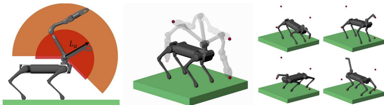
Fig. 2 Visualization of the range of motion for the proposed one-DoF robotic arm mounted on Unitree Aliengo. On the left, a geometric representation shows the range of motion in the sagittal plane over the angle of arm elevation. In the center, the six-DoF arm can reach all four points in space without the robot moving. On the right, an example of the equivalent poses the robot equipped with the one-DoF arm can achieve to reach the same points in space.
