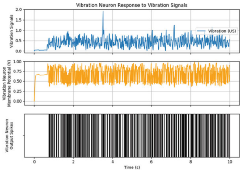
Fig. 15.6 Vibration neuron response to acceleration
