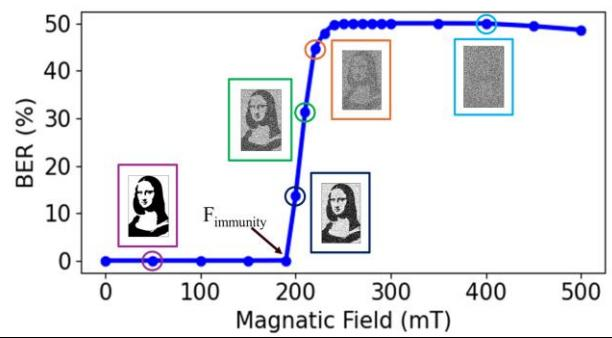
magnetic field beyond the standby immunity threshold leads to a significant spike in bit flips. This is likely attributed to the coercive field, which represents the barrier between two logical states (see Fig. 1(d)), influences the MTJ magnetization switching process [16]. Consequently, even minor magnetic field changes can induce substantial bit state transitions, which persist at higher fields.
