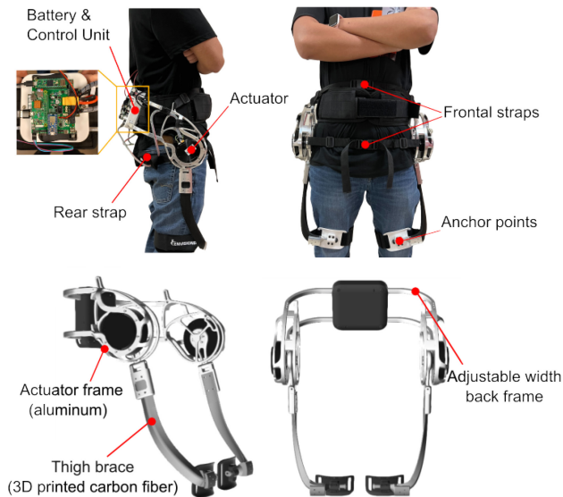
Fig. 1. Our new proposed portable hip exoskeleton consists of two quasi-direct-drive actuators, adjustable width back frame, multi-strap wearable, and compact electronics. This design reduced wobbling (relative angular velocity between the human and robot) by 74% compared to a traditional configuration.
