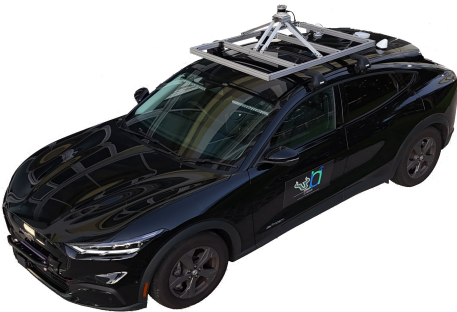
Fig. 1: The RANCS lab EV, equipped with sensors for real-time data collection.
