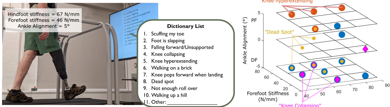
Fig. 7. Experiment 2. Left: Subject walks on the treadmill while looking at a dictionary of possible sensations. Each combination of forefoot stiffness (3 levels), hindfoot stiffness (3 levels), and alignment (3 levels) was tested once, and the subject was asked which phrase best described their sensation. Right: Location of patient sensations relative to forefoot stiffness, hindfoot stiffness, and dorsi/plantarflexion alignment.
