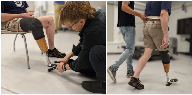
Fig. 5. Left: Certified Prosthetist adjusting the Footropter while the subject is seated. Right: Example of a trial, in which the subject walks overground with the Footropter and provides binary feedback on their preferences.
