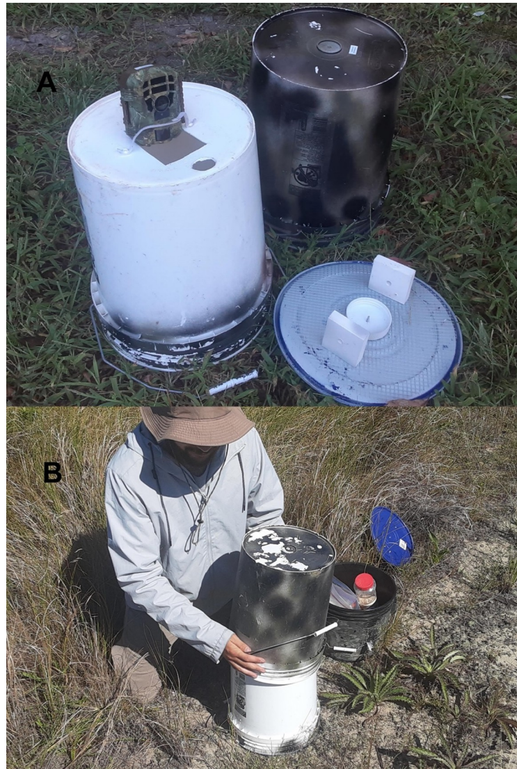
Fig 1. The MouseCam. A) Parts of a MouseCam including the inner bucket (left), with 4.5 cm holes near the rim to allow animal access, and an opening in bottom of the bucket for the trail camera to be attached facing down, with a Velcro strap to secure it; the lid (lower right), equipped with a reservoir for bait, and “walls of despair” to frustrate predators attempting to access the bait; and the outer camouflage bucket (upper right). B) deployment of a MouseCam. The outer camouflage bucket provides protection for the camera within. It is secured to the inner bucket with a self-tapping hex screw. The bails of both buckets are attached to the ground using anchoring stakes.
