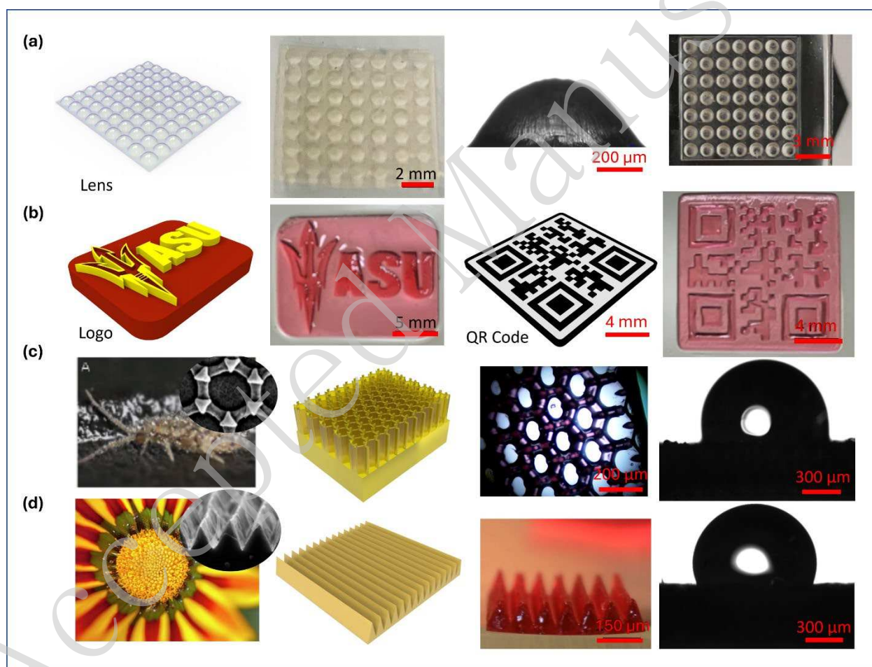
Fig. 4 Macro and Micro-scale fabrication results (a) Designed CAD model, printing results and side view microscope image and demo test of transparent lens array; (b) CAD model and fabrication results of ASU logo and QR code; (c) Hierarchical surface structure of springtails (Collembola), CAD model of biomimetic structure, microscope image of fabrication results and
