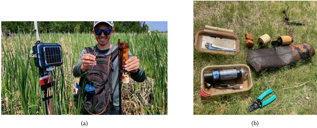
Fig. 3. (a) Spudnik that failed from beaver chewing its wires (b) Onset HOBO datalogger after being removed from the sandy river
