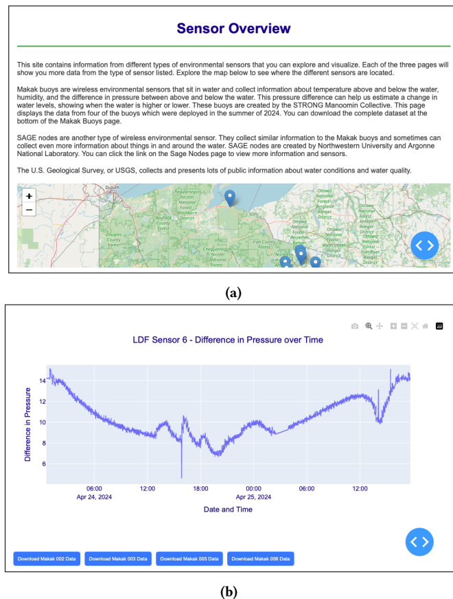
Figure 8: The LDF temporary sensor dashboard. (a) the home page of the dashboard, with descriptor text and a map of sensor locations. (b) An example graph from the Makak sensor showing the difference in air and water pressure.
