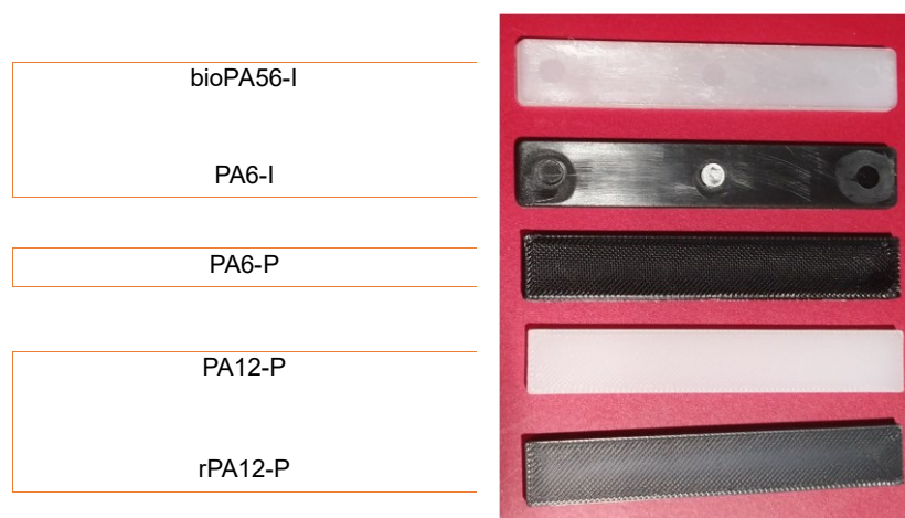
Figure 4: Polyamide specimens used in water absorption experiment.
