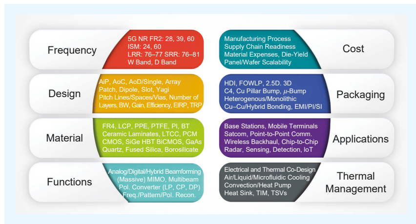
FIGURE 8. Guidelines for developing antennas in the mm-wave band. NR: New Radio; BW: bandwidth; EIRP: effective isotropic radiated power; TRP: total radiated power; PPE: polyphenylene ether; HBT: heterojunction bipolar transistor; MIMO: multiple-input, multiple-output; freq.: frequency; satcom: satellite communications; EMI: electromagnetic interference; PI: power integrity; SI: signal integrity; IoT: Internet of Things; LRR: long-range radar; SRR: short-range radar; PTFE: polytetrafluoroethylene; BT: bismaleimide triazine; LP: linear polarization; CP: circular polarization; DP: dual polarization; HDI: high-density interconnect; Recon.: reconfigurability; Comm.: communication.
