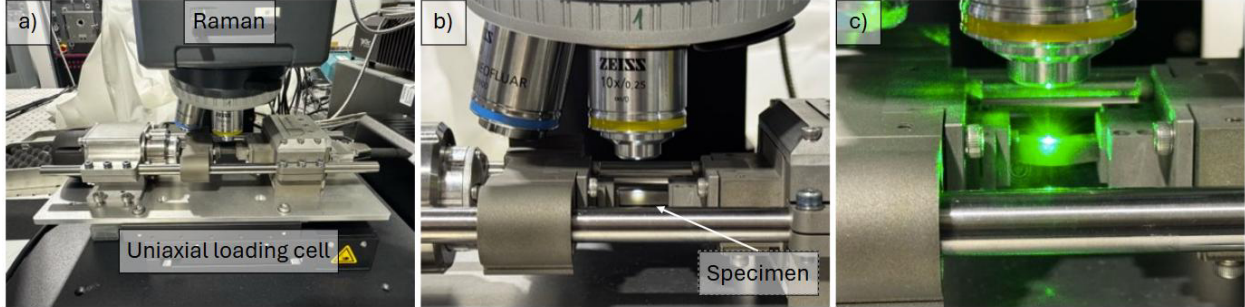
Fig. 1 a) Experimental setup with Raman and light microscope function, equipped with uniaxial loading cell; b) High magnification of experimental setup with mounted specimen in uniaxial loading cell; c) Loaded specimen exposed to a 532 nm laser
