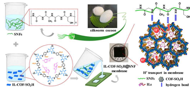
Fig. 23 Schematic illustration of preparing of the IL-COF-SO 2 H@SNF composite membrane. (Reproduced from ref. 173 with permission from Elsevier.)
