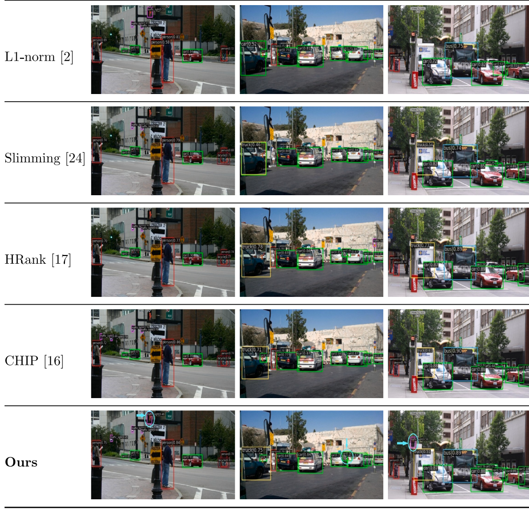
Fig. 5. Qualitative results of competing SOTA approaches (i.e., L1-norm pruning [2], Net Slimming [24], HRank [17], and CHIP [16]) and our method on example images from COCO_traffic. In each case, the detection image was produced using YOLOX-S pruned at a 40% pruning rate on COCO_traffic. The final row highlights cyan circles, indicated by arrows, demonstrating the superior performance of the detector pruned using our approach over other competing methods. Best viewed when zoomed in.
