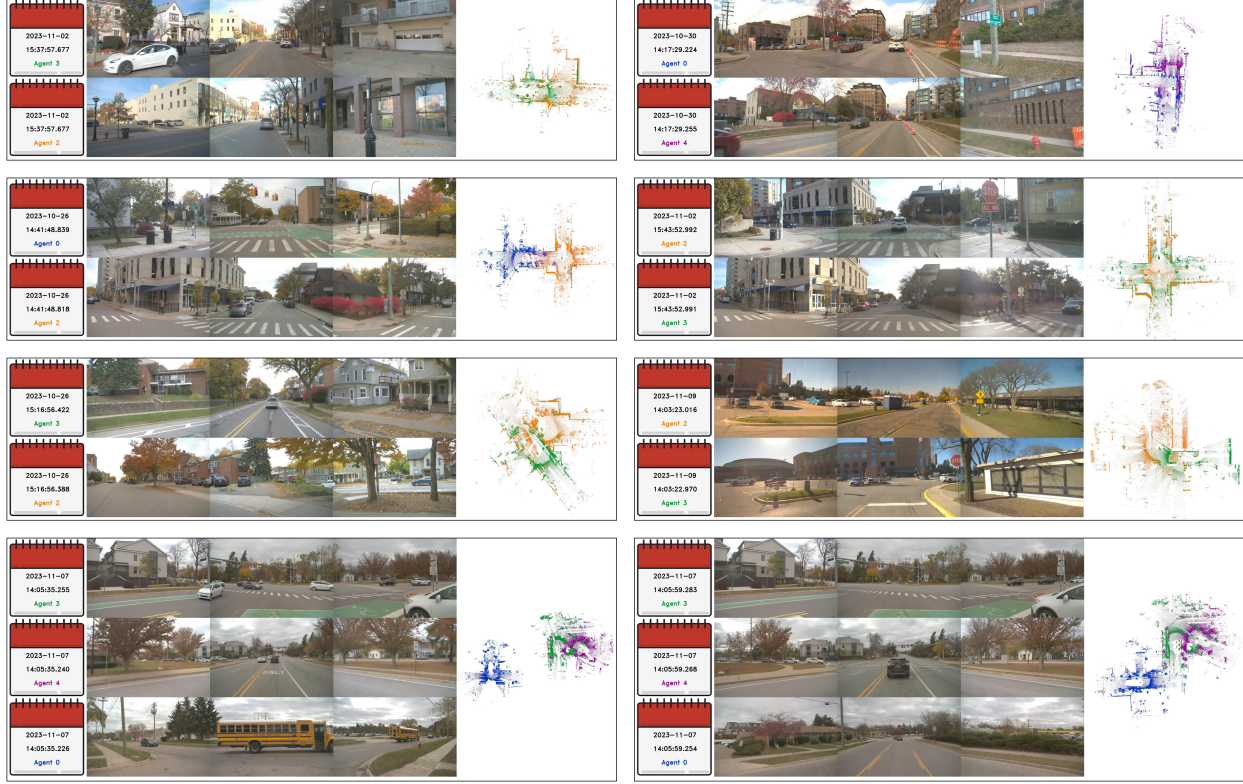
Figure 7. Multiagent scene visualizations with three front cameras and LiDAR point clouds in bird's eye view (BEV). Typical scenarios include straight road tailgating as well as meeting at intersections.
