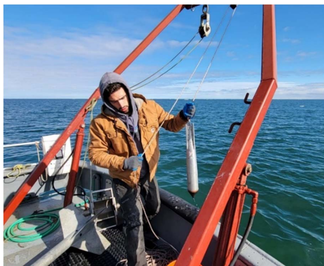
Fig. 2. PFFP, blueDrop, in use during the field survey in Harrison Bay. (Image by Nina Stark.)
