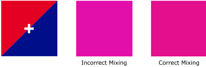
Fig. 2. Mixing of red (sRGB [227, 0, 34]) and blue (sRGB [0, 15, 137]) lights in the non-linear sRGB space (incorrect) vs. in a linear color space (correct).
