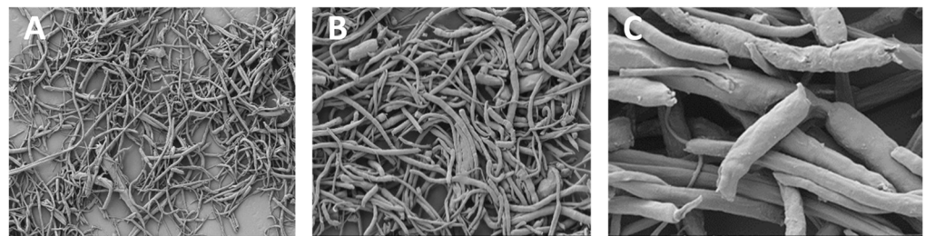
Figure 7. SEM images of cryoground PG nanofibers under (A) 500 X magnification and a scale bar of 20 µm; (B) 1.00 KX magnification and a scale bar of 10 µm; (C) 5.00 KX magnification and a scale bar of 1 µm.
