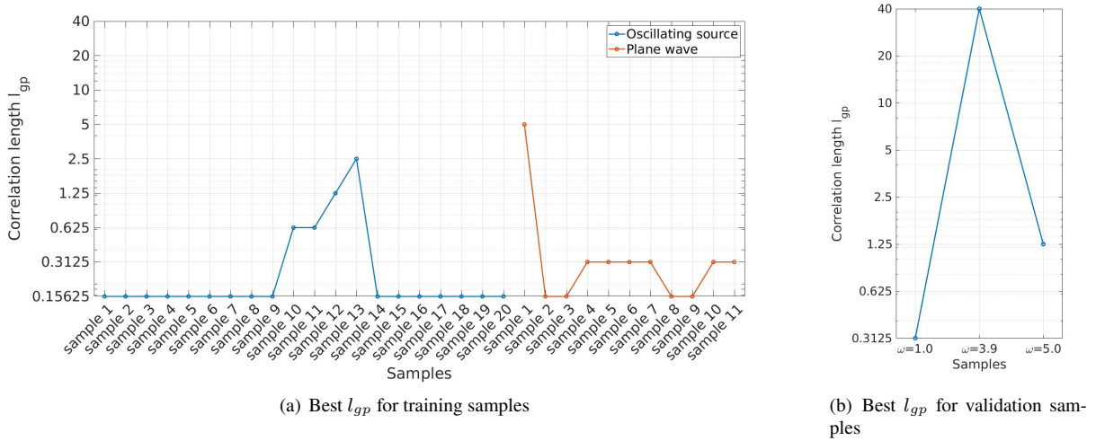
Fig. 10. Best l_{gp} (with the lowest CRPS) on training and validation samples for a bar with periodic material.
