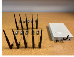
Fig. 3. LoRa transmitters and a USRP receiver.
