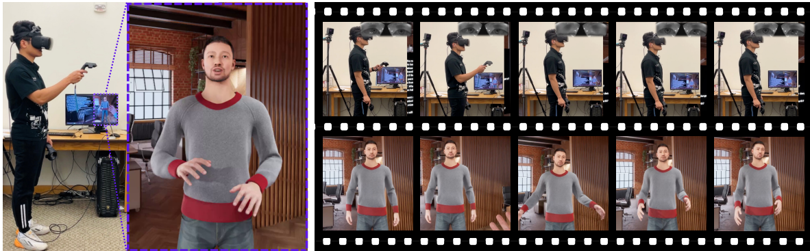
Figure 1: With our method, VR users can interact with a virtual agent naturally through a combination of multiple modalities including verbal expressions, body language, and eye contact. In the right, the top row shows a VR user's multi-modal behaviors while he interacts with a virtual agent; the bottom row shows the agent's real-time reactions.
