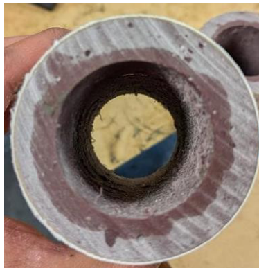
Figure (2): Cross-Sectional view of Ablative Liner
