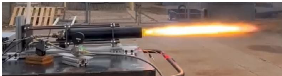
Figure (5): Hot-Fire at 300 psi Fuel Pressure for 60/64" Nozzle
