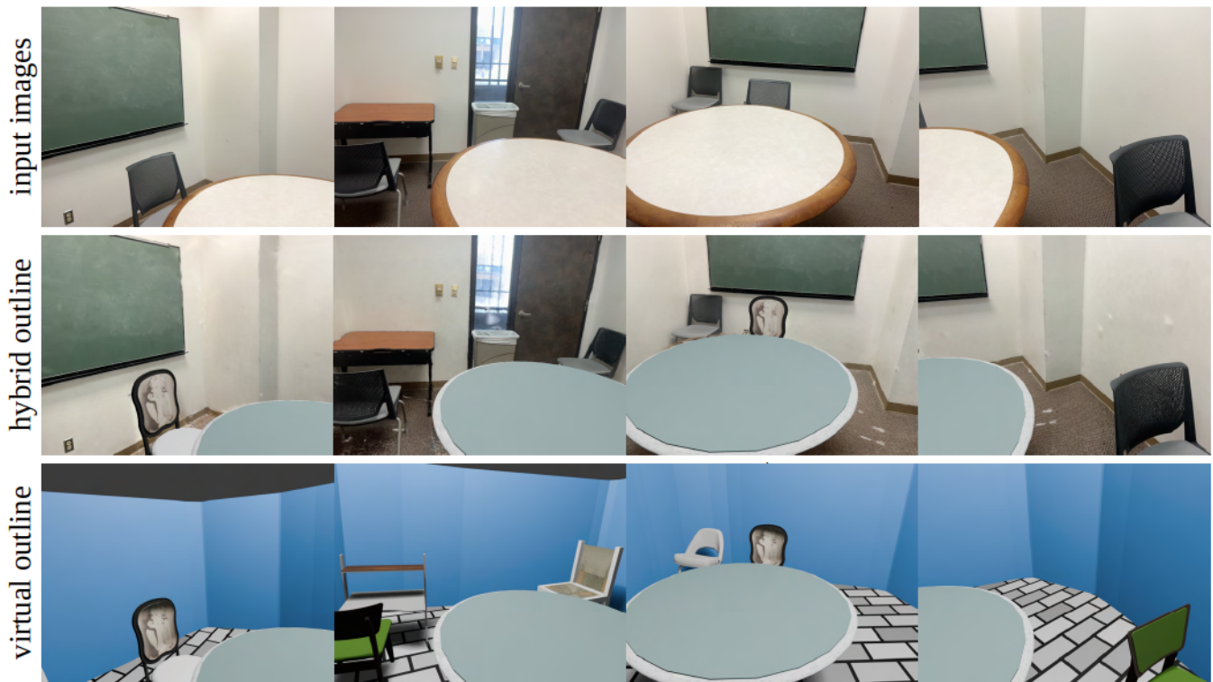
Figure 4: This illustration shows the design results from our automated pipeline. (Top row) The captured input image; (Middle row) The hybrid outline, which includes both the reconstructed gaussians and CAD models; (Bottom row) The virtual outline, where all elements are replaced by the CAD model.
