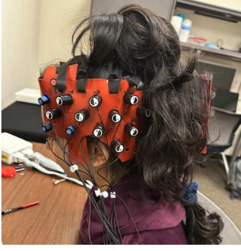
Figure 2: Image of our fNIRS cap on a participant. The cap goes around the head covering frontal and temporal regions.
