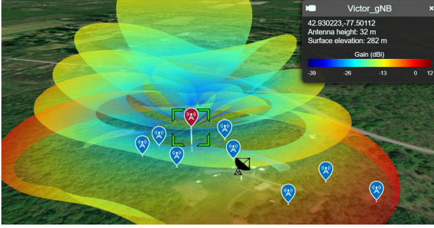
Fig. 4. Radiation pattern of the gNB when using our heuristic solution. The red pin indicates the location of the simulated gNB, the black telescope is the RAS, and the remaining blue pins are the locations of simulated UEs.
