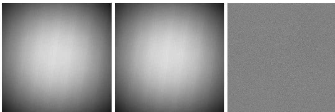
Figure 2. Air X-ray images ( left and middle ) used to derive the noise profile ( right ).
