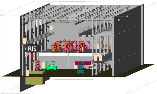
Fig. 2. Indoor factory environment in Wireless-Insite. The BS is located on the ceiling, while the RIS is mounted on the wall. The RIS is represented by the red hemisphere on the left wall.
