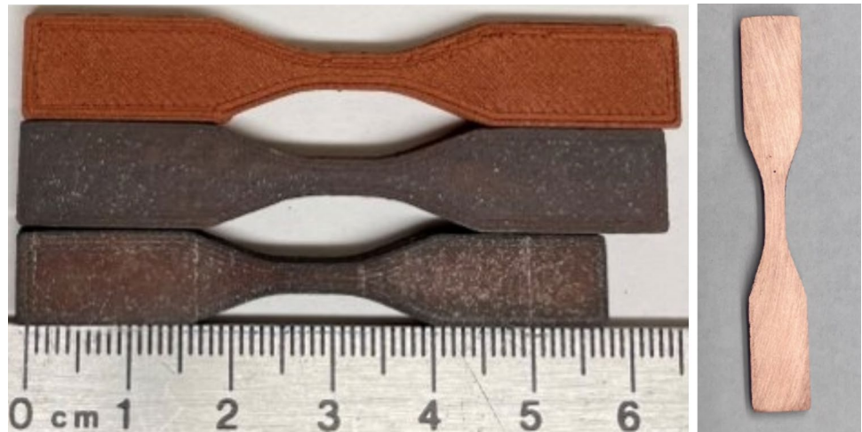
Fig. 7 Dog bone sample shrinkage example, (top) green, (middle) brown, (bottom) control sintered, along with (right) polished dog bone sample(not to scale)
