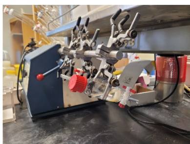
Figure 6. A) SPPS flow chart of compound 13; B) resin swelling, 1 st amino acid loading, capping, and cleavage are performed by shaking; C) amide coupling and Fmoc removal reaction are stirred by bubbling; D) liquid phase is pushed out of the SPPS vessel with air or nitrogen to separate it from beads.
