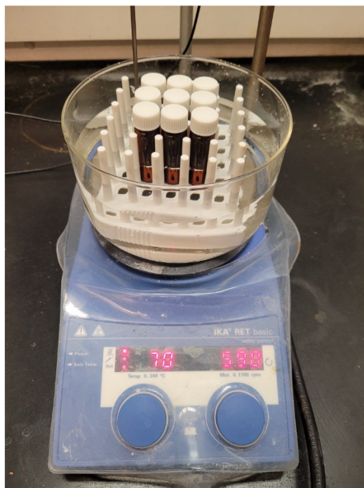
Figure 4. A) Synthesis of compound 15 ; B) aerobic cross-dehydrogenative coupling set ups.
