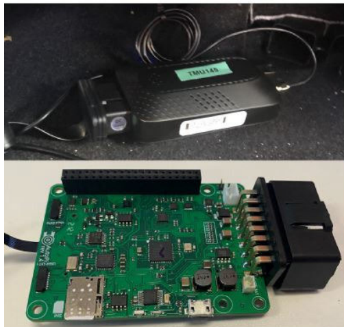
FIGURE 10. Overview of the Raspberry-based TMU [27].
