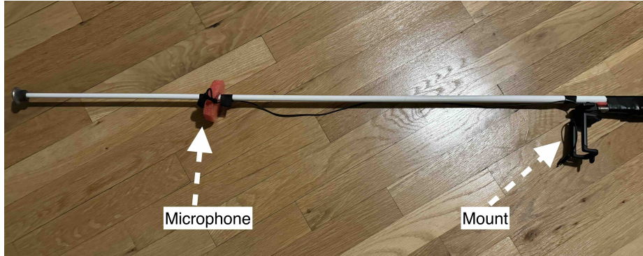
Fig. 1. The modified white cane for sidewalk material audio data collection.
