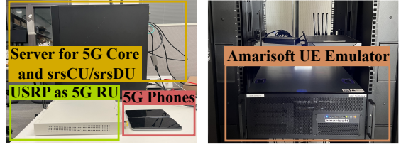
Fig. 8— Hardware used in L4Span implementation. One desktop server runs the 5G Core, srsCU and srsDU, and the USRP is served as the RU. We use both real phones and Amarisoft UE emulator as the UEs for the evaluation.
