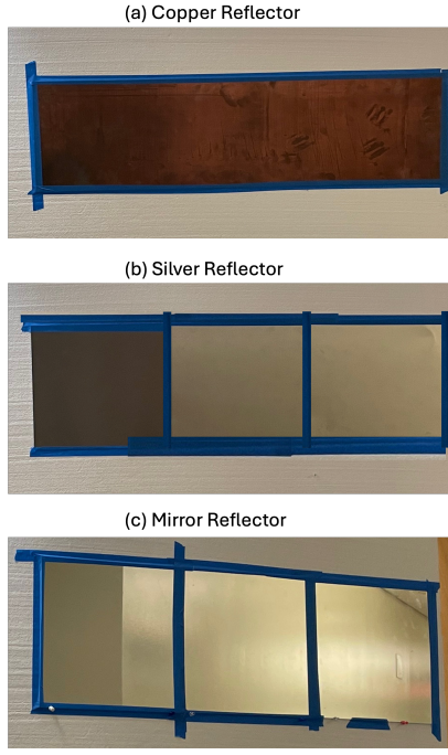
Fig. 4. Flat passive reflectors of size 0.3 \times 0.9 \text{ m}^2 mounted on a foam board at an azimuth angle of 45^\circ with respect to the transmitter.
