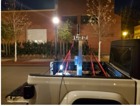
FIGURE 6. RX of the ReRoMA sounder loaded on the back of the pickup truck.
