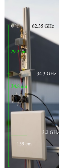
Fig. 3. Receive antennas mounted on a pole of a tripod [2].
