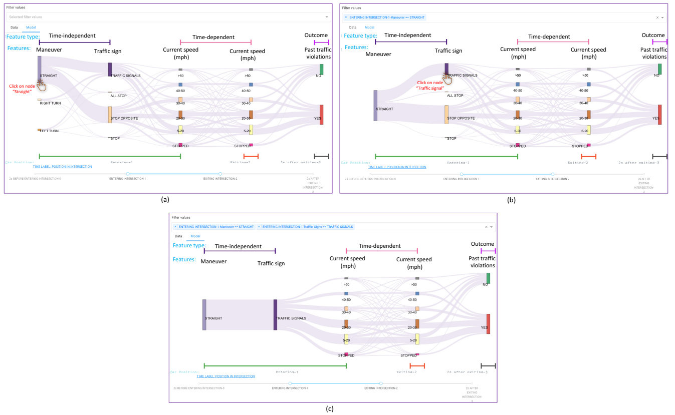
Figure 4: Interactive filtering of feature values to create a “what-if” scenario when drivers went straight through traffic signals: a) before filtering, b) after filtering “Maneuver” is “Straight”, and c) after further filtering “Traffic sign” is “Traffic signals”.
