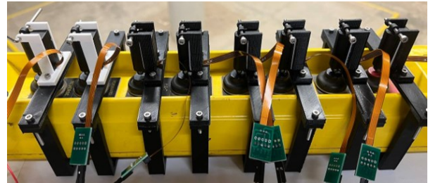
Figure 6. Crane remote control with mounts and actuators.
