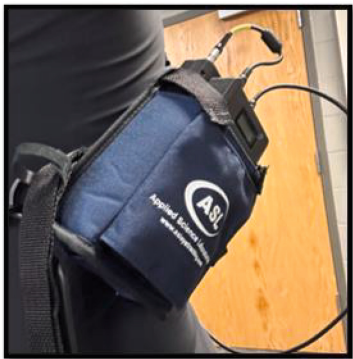
Fig. 3. Powering unit for the Eye Tracker hung across the body.
