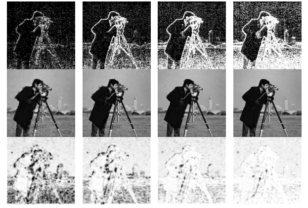
Fig. 3: Performance of the proposed method with different error threshold \Delta : (Top) Selected Pixels (white) using Predictive Sampling; (Middle) Reconstructed image; (Bottom) SSIM map of the reconstructions in contrast with the original image.
