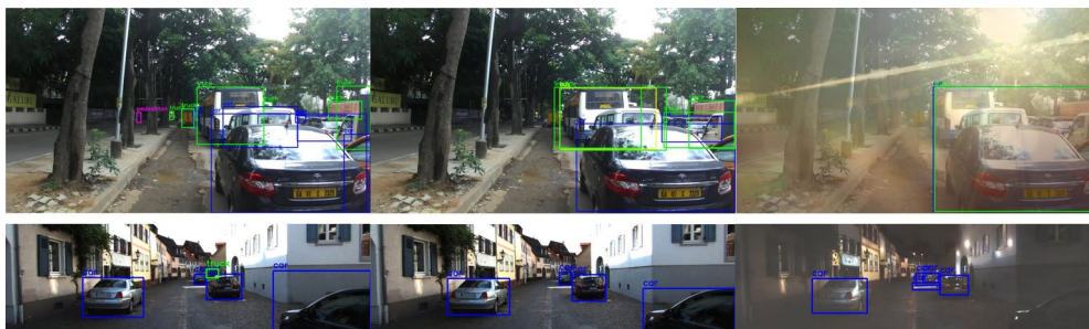
Fig. 1 Object detection model, i.e., DETR [1] fails to detect objects accurately under weather challenge (left: original images with ground truth, middle: original images with DETR detections, right: weather synthetic images with DETR detections)
