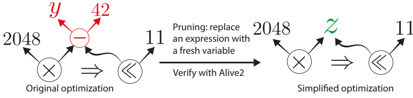
Fig. 2. Pruning an optimization. (y - 42) is replaced with the fresh variable z that can match any expression. A subtraction of 42 is no longer necessary for the optimization to apply.
