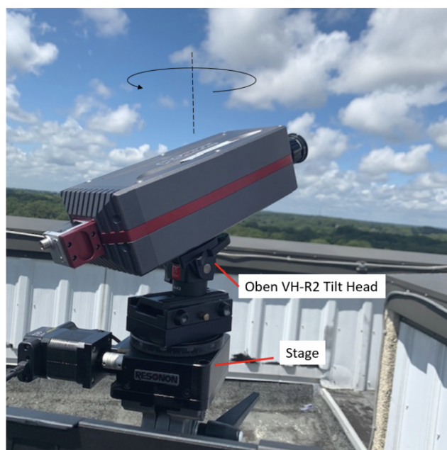
Figure 2. Resonon Pika XC2 camera mounted on a tilt head and attached to a rotational stage that captures sky images covering a 90-degree range in azimuth [12].
