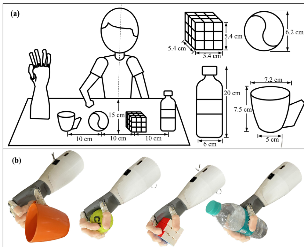
Figure 2. (a) Experimental setup and dimension of the grasping objects. (b) Grasping of four objects by ENRICH.
